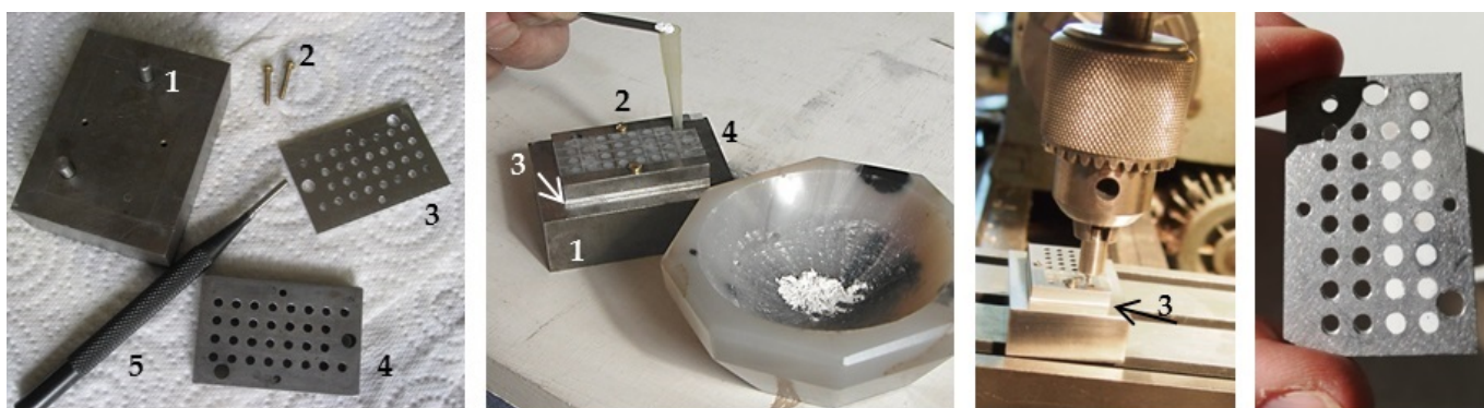
Sample preparation sequence for CL-quantitative analysis developed by Ph. Blanc at UPMC, Paris (© Ph. Blanc)
