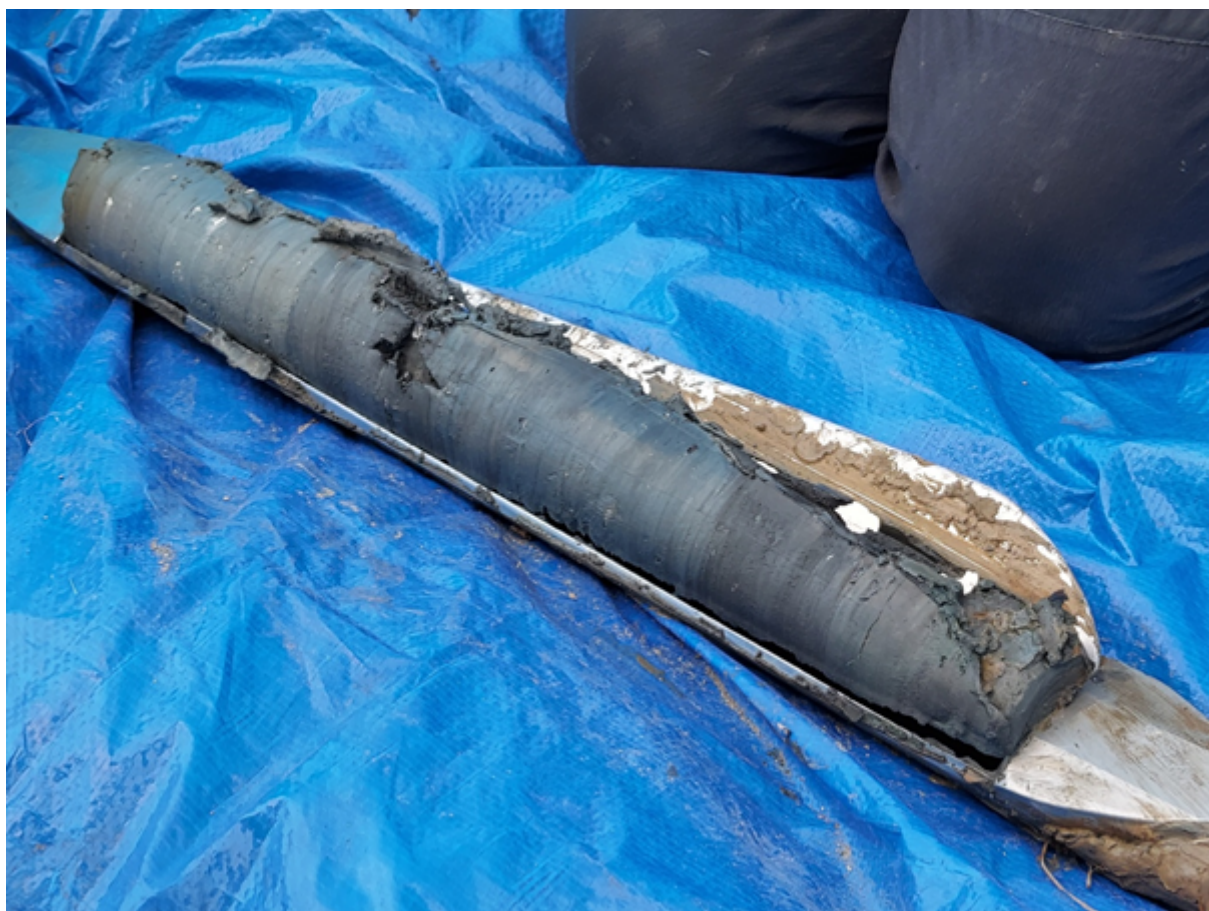
The Russian corer head full of lagoon sediments (and of palaeoenvironmental information!). Photo: GIAP/ICAC
