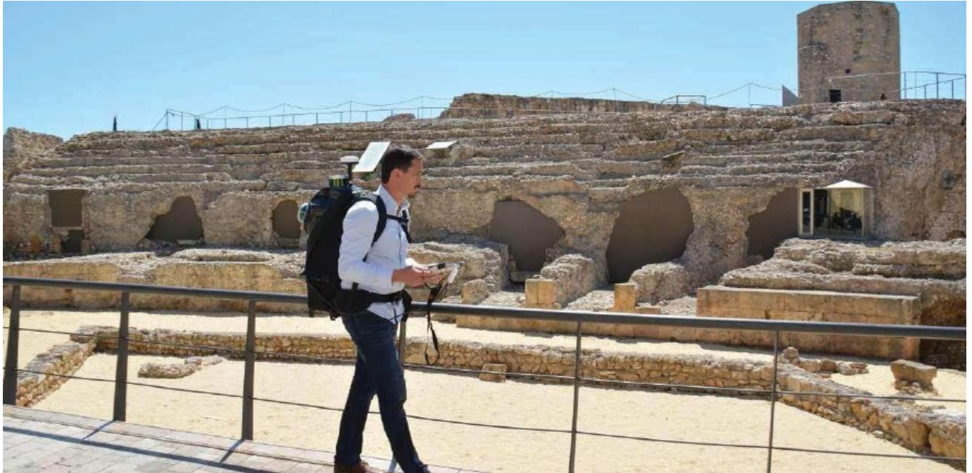
Scanning (backpack laser) in the Roman Circus of Tarragona. Photo: ICAC.
